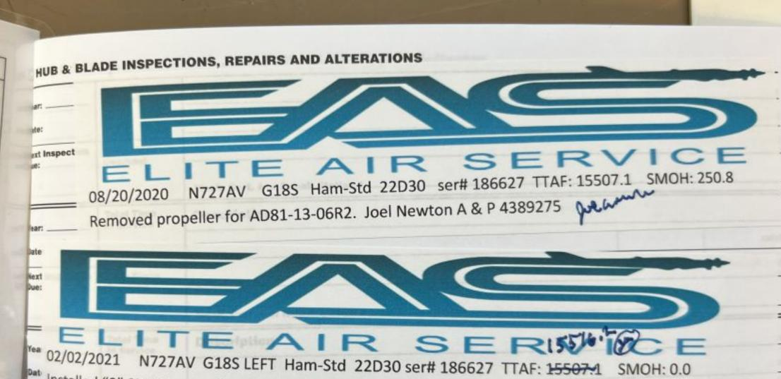
Installed "0" SMOH propeller on Left engine. Beech service manual 414-180161 B10 2797 and Hamilton
