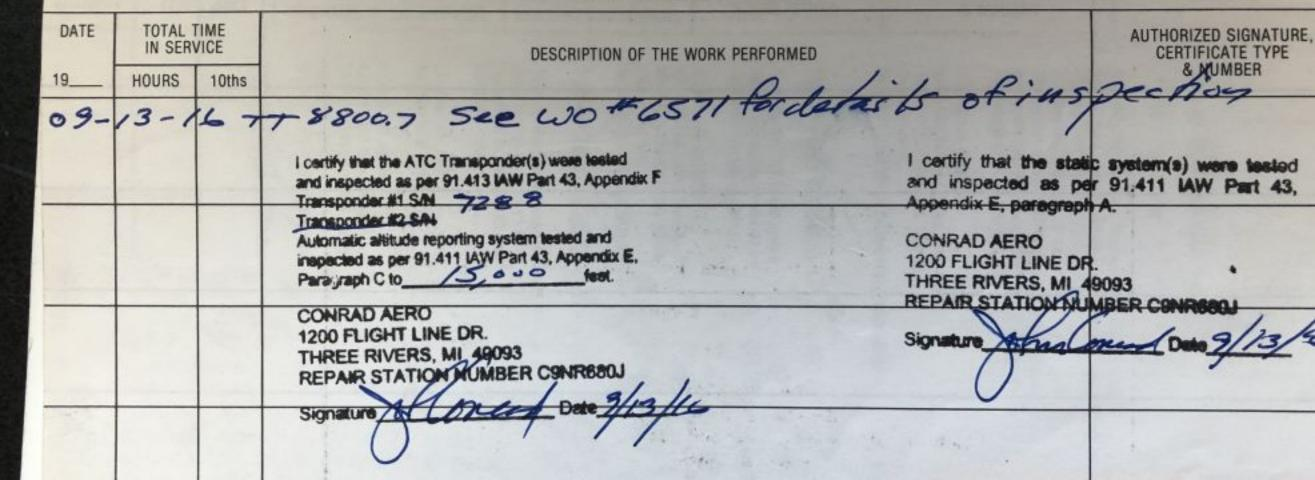
N9208U Cessna 150M SN 15078159 Tach time 8803.2 TTSN 8803.2 Airframe annual inspection completed per Cessna 150M inspection guide. AD's checked with none due at this time. Complied with AD 80-11-04, 11-10-09 Replaced ELT battery Due 11-2018, Inspected and tested per FAR 91.207 Inspected cables, pullys, serviced brake master cylinder. This airframe has been inspected and found to be in airworthy condition
